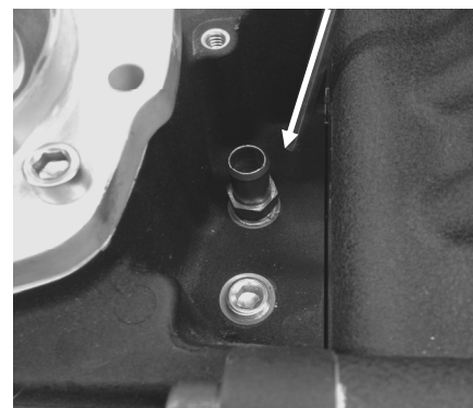
STRAIGHT FITTING INSTALLED. FIGURE 2
