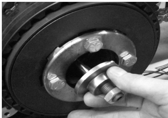
INSTALLING KEYHOLE FITTING| FIGURE 5
